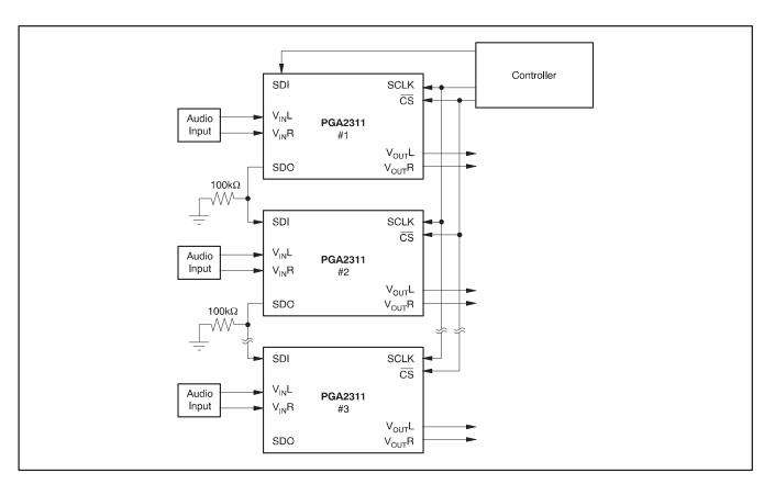
Figure 4. Daisy-Chaining Multiple PGA2311 Devices.
