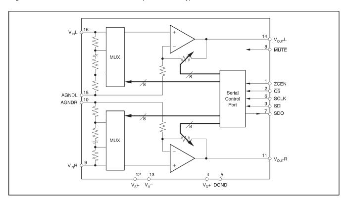
Figure 1. PGA2311 Block Diagram.
