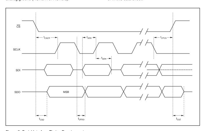
Figure 3. Serial Interface Timing Requirements.
